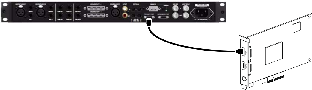
Figure 3. HD OMNI connected to the DigiLink Mini Port 1 on an HD Native card (8-channel system)
